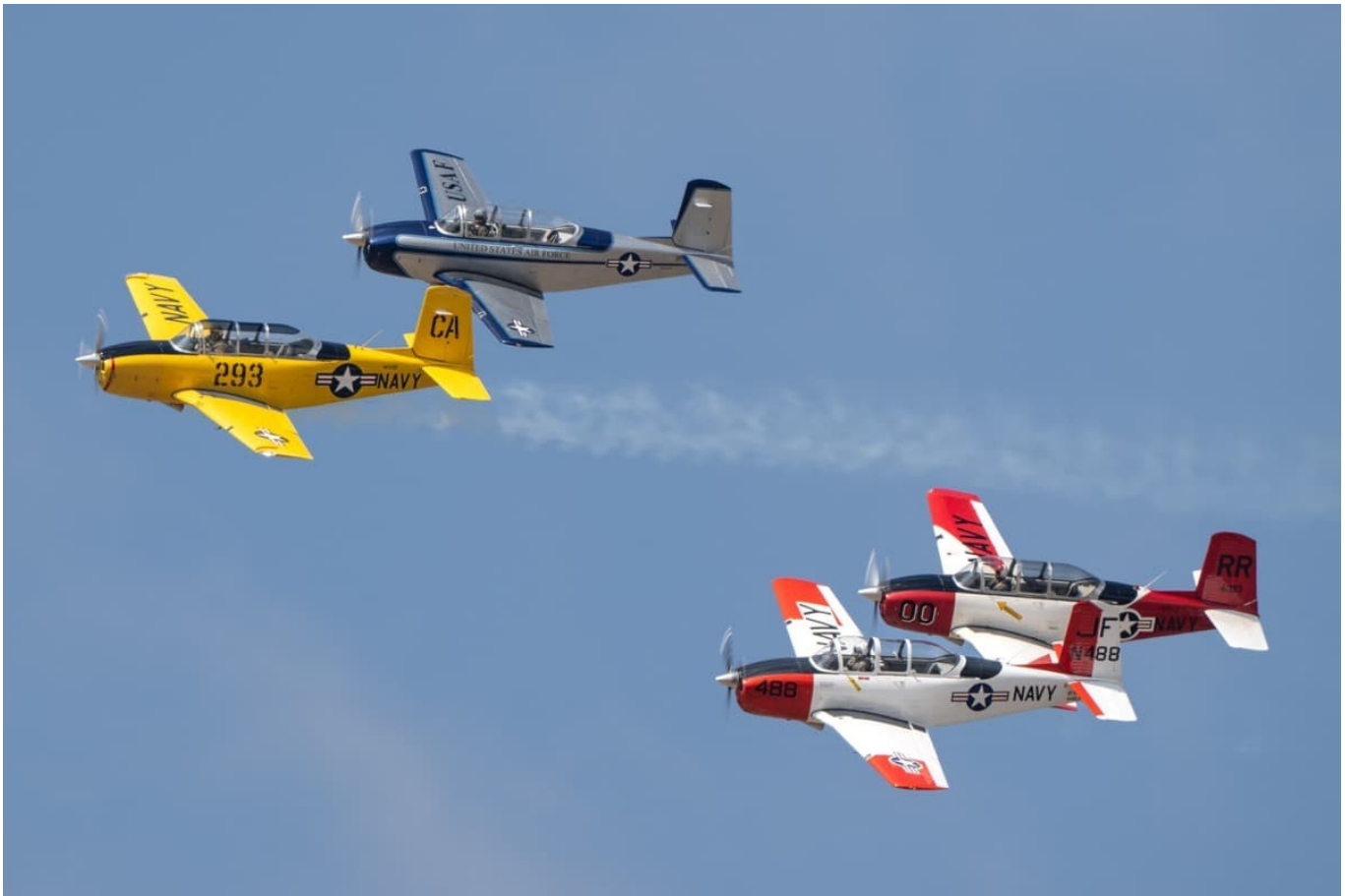
A quartet of T-34 Mentors perform during the air show. The T-34 Mentor was a military adaptation of the Bonanza Model 35 design, capable of +10g and -4.5g loads.
